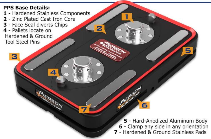
**PPS Pallets** - Four pallet sizes range from 8"x12" to 10"x16" and locate with .0003" repeatability. 6061-T6 Extruded Aluminum assures easy machinability. The bottom locking surfaces use hardened stainless steel components for long life.
